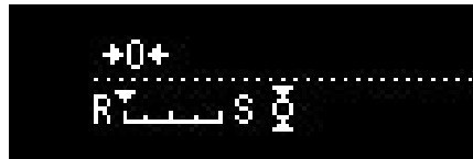
Moving it left prioritizes response and moving it right prioritizes stability. Five setting levels are available.
