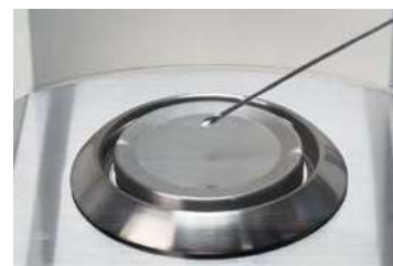
Measurement values change when an electrically charged measuring spoon is simply moved near the sample
