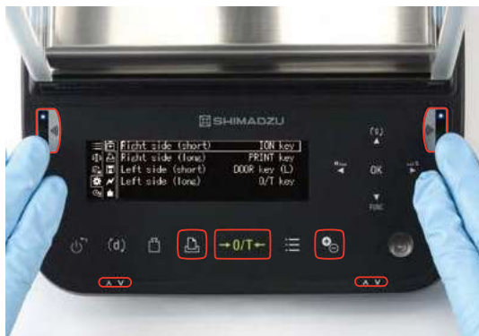
Checking the status of function settings by holding hands over both touchless sensors
