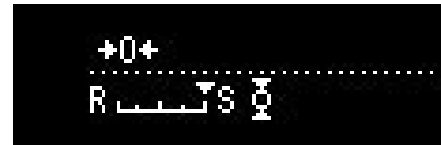
Moving it left prioritizes response and moving it right prioritizes stability. Five setting levels are available.
